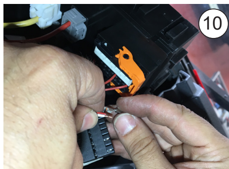
Fasten the cables in the supplied terminal
